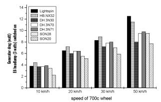
Fig. 4: Nighttime resistance (light on). SON20 is most efficient.
